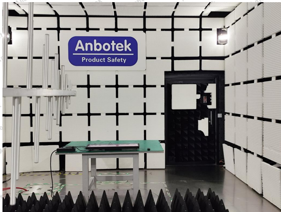
Photo of RF Field Strength Immunity Test
